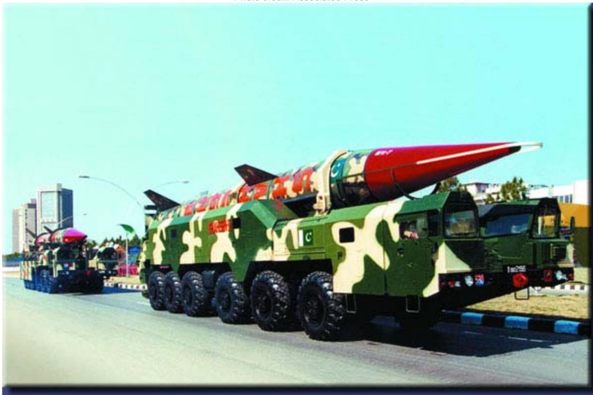
Pakistan's new two-stage, solid-propellant Shaheen II MRBM was publicly displayed for the first time in the Pakistan Day parade in March 2000. The missile, which has not yet been flight-tested, could have a range of 1,250 miles or more, in the same class as India's new Agni II MRBM. The chassis for the launcher (front vehicle) and missile transporter (rear vehicle) were produced in Belarus by MAZ, which also produces the launcher chassis for the Russian SS-25 and SS-27 ICBMs.
