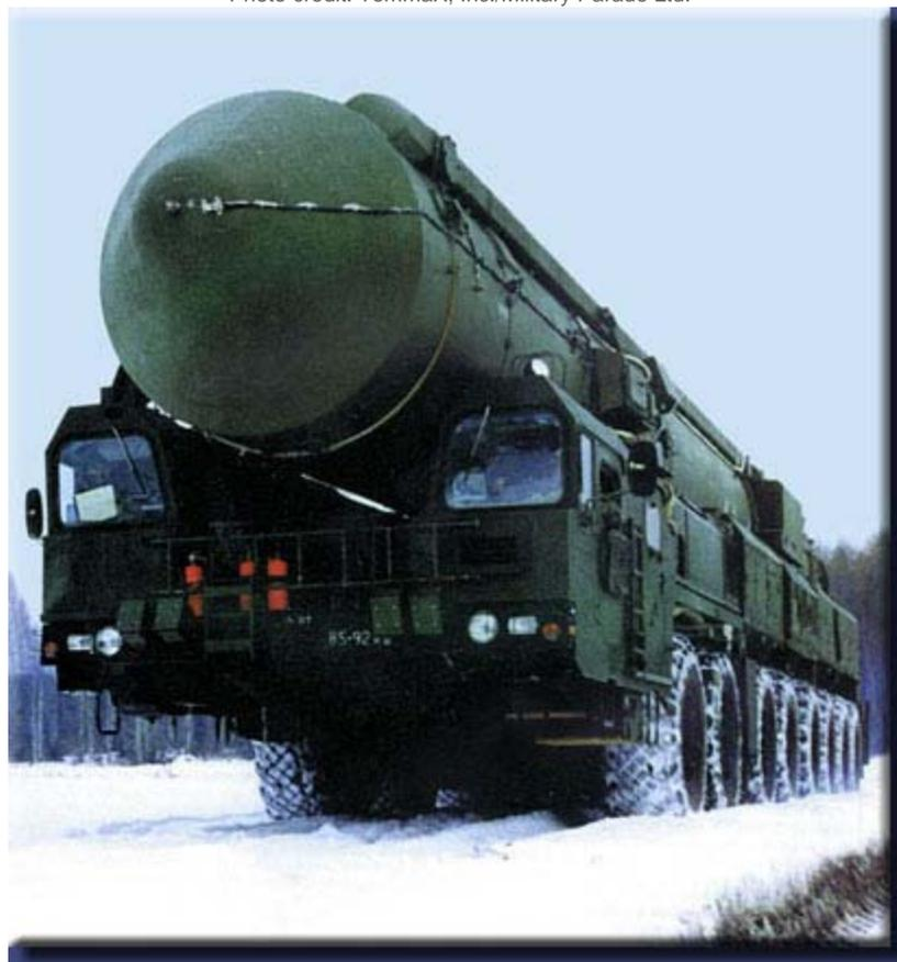
The road-mobile SS-27 ICBM will be carried in a canister on a new eight-axle transporter-erector-launcher.
