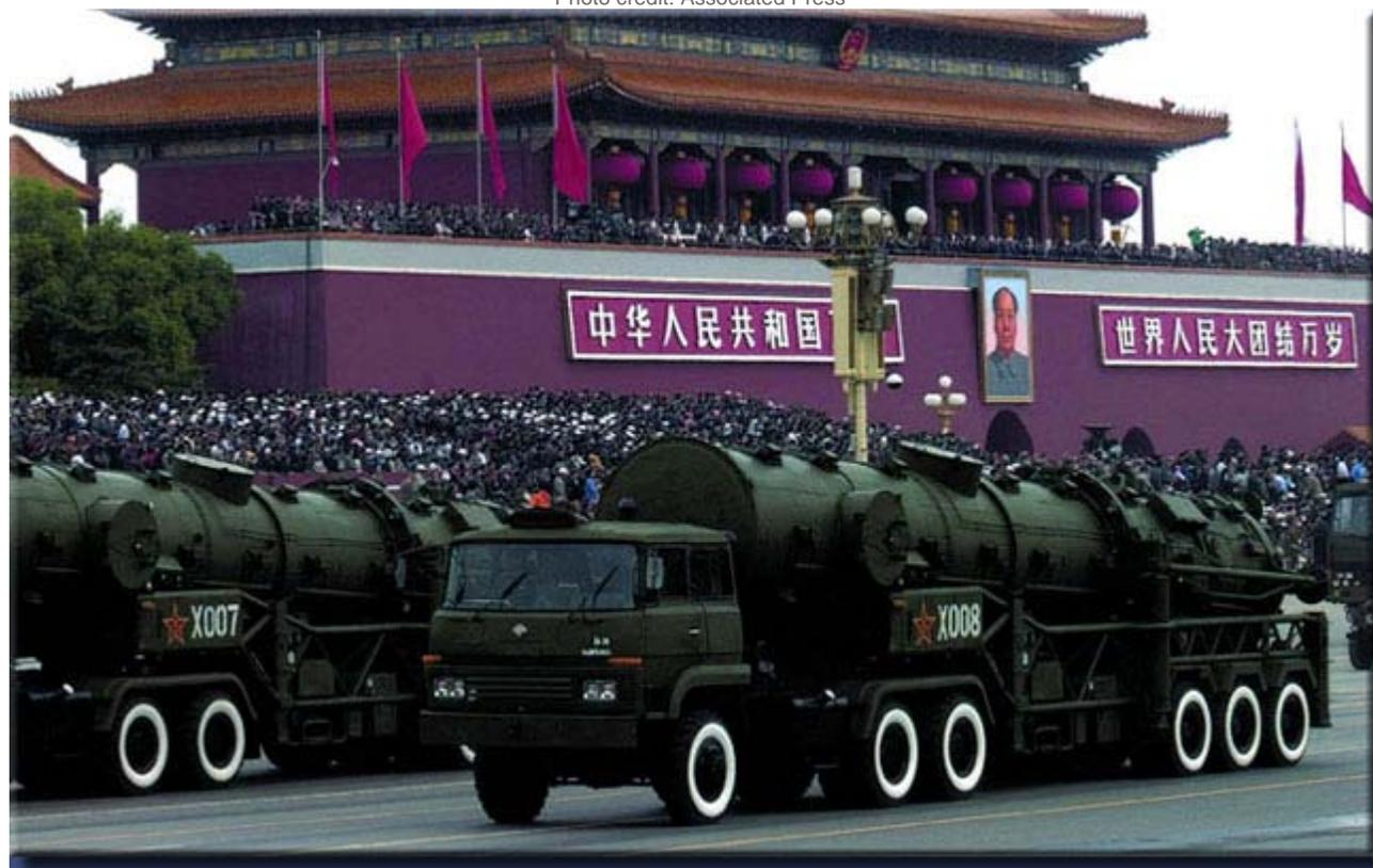
The CSS-5 is a two-stage, solid-propellant MRBM capable of reaching targets in the Pacific theater and most of Asia. The missile is carried in a canister on a towed erector-launcher.
