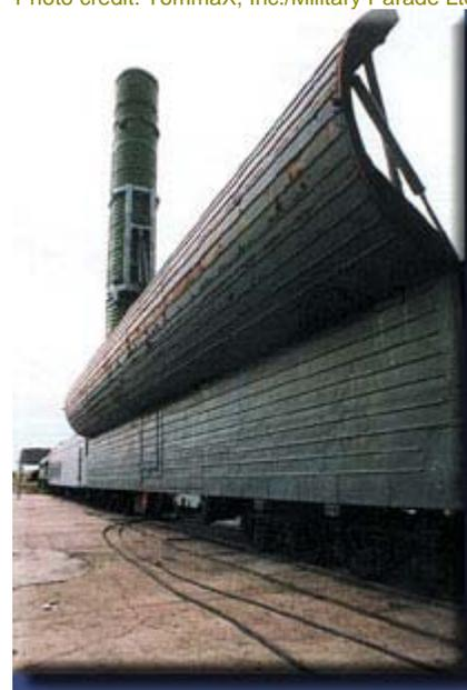
SS-24 Launcher and Launch Canister
