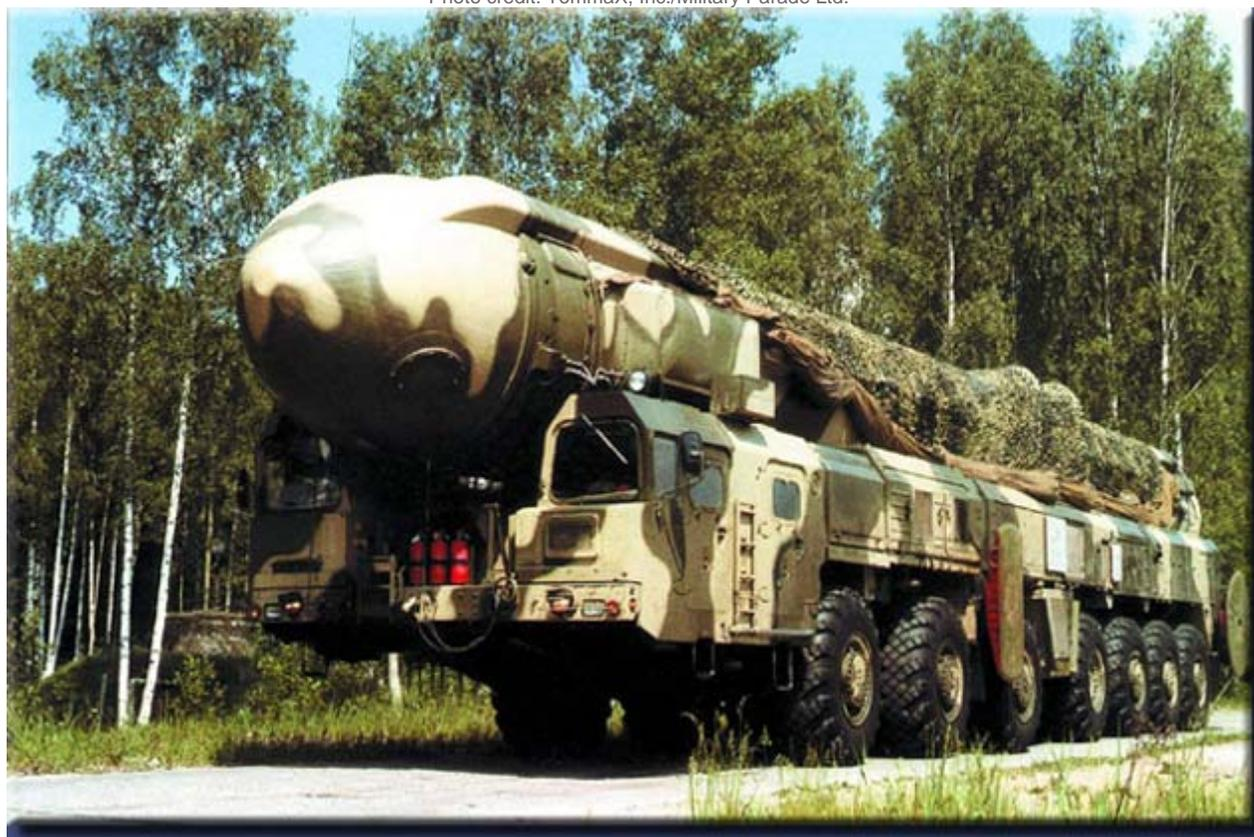
There are 360 SS-25 missiles deployed, more than any other type of foreign ICBM. The missile is launched from a canister carried on a seven-axle transporter-erector-launcher.
