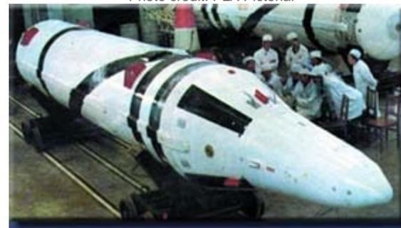
The CSS-NX-3 SLBM is a two-stage, solid-propellant missile.
