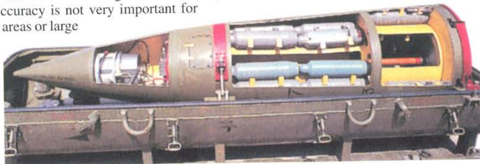
Ballistic Missile Warhead with Submunitions
