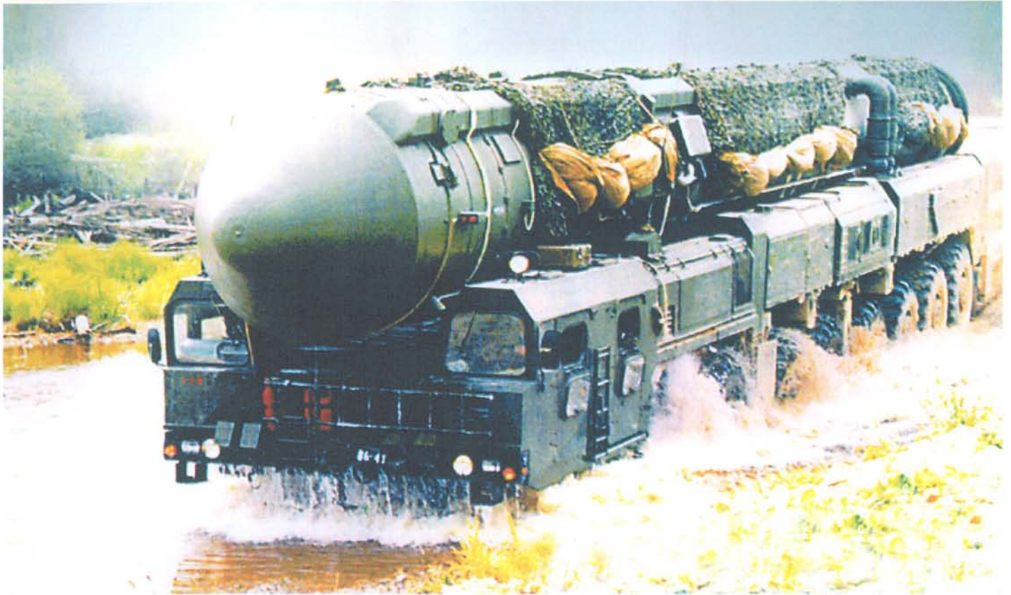
Russian Road-Mobile SS-27 ICBM on its Transporter-Erector-Launcher
