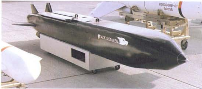
The Black Shaheen is an export version of the French SCALP-EG cruise missile.
