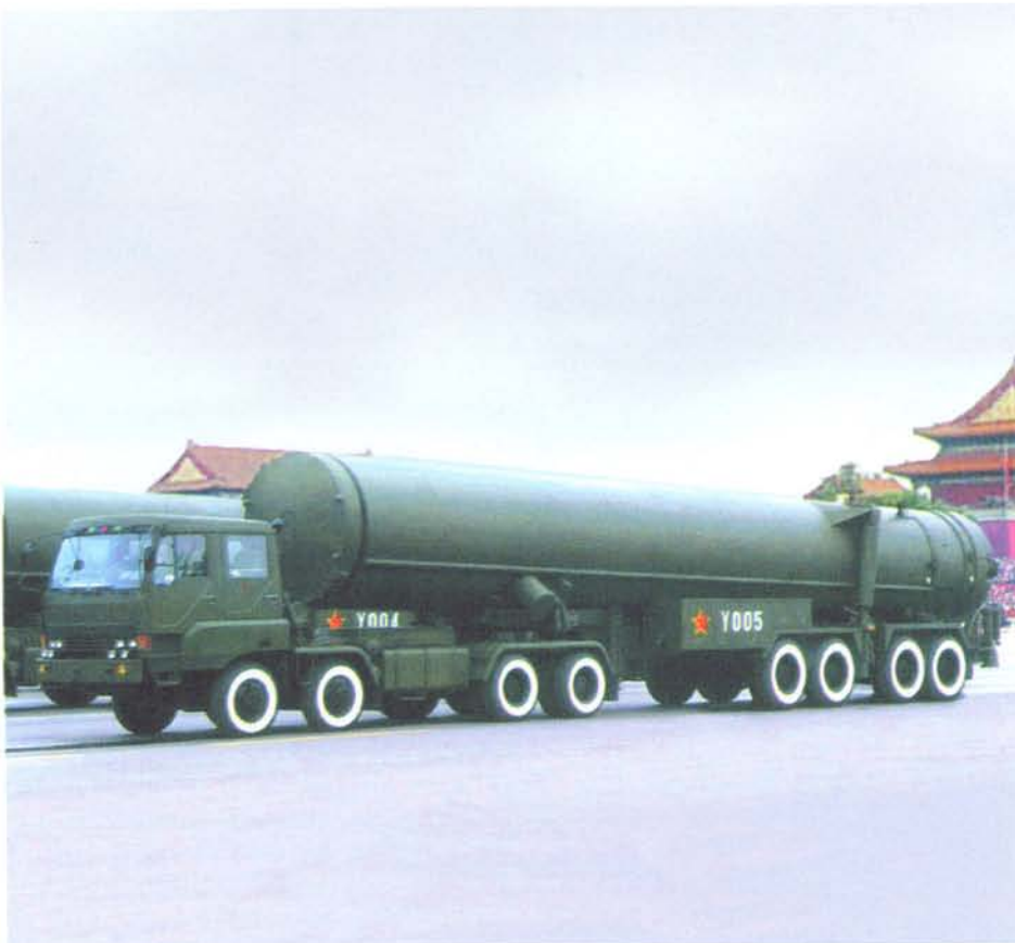
China is continuing development of the new DF-31 road-mobile ICBM (a three-stage, solid-propellant missile carried inside a canister).
