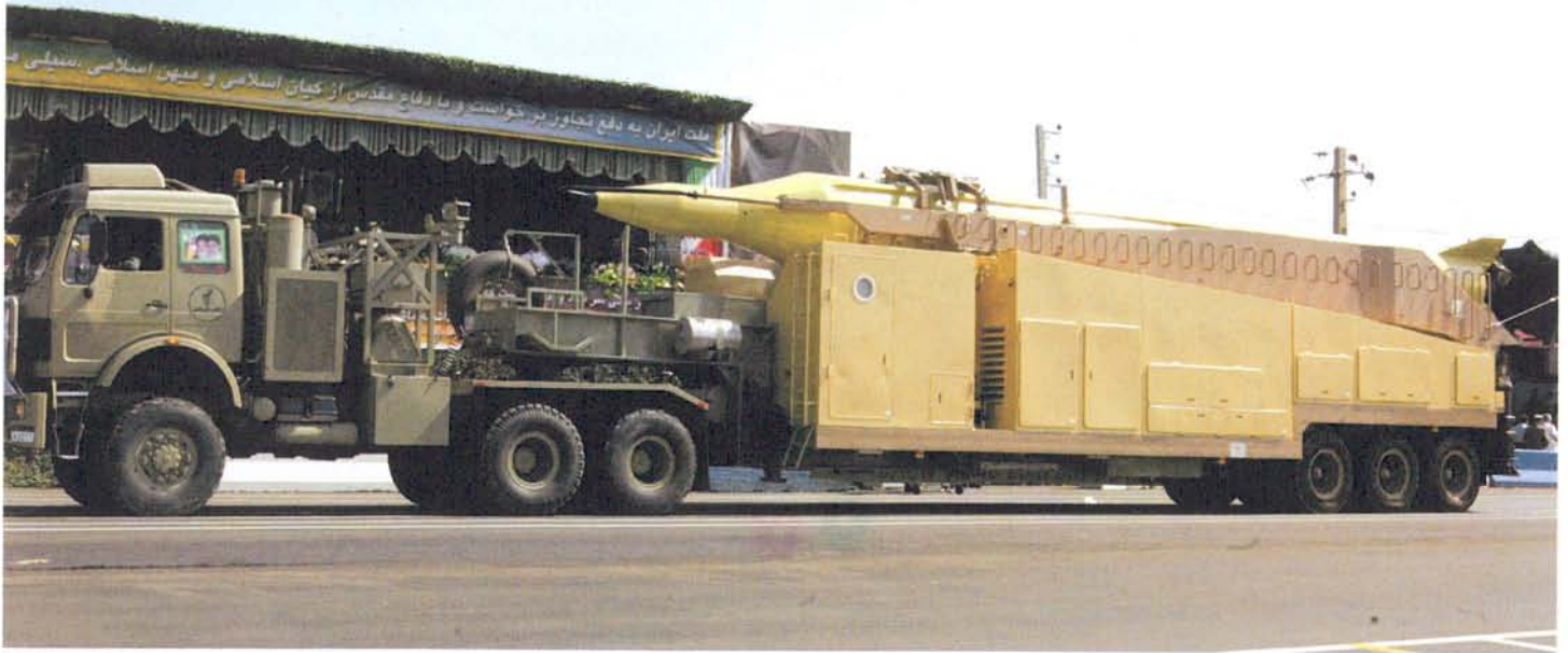
The Iranian Shahab 3 is a single-stage, liquid-propellant missile based on the North Korean No Dong MRBM.
