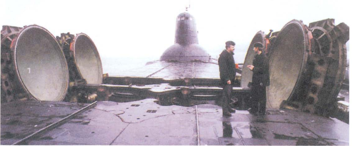
Russian TYPHOON SSBN with Launch Tube Doors Open
