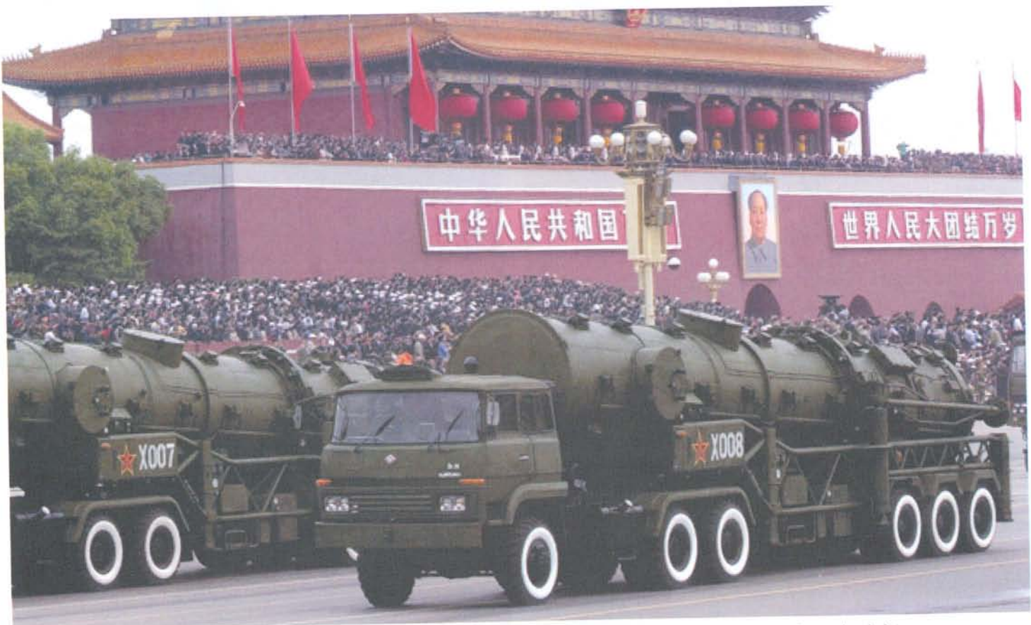
The Chinese CSS-5 is a two-stage, solid-propellant MRBM capable of reaching targets in the Pacific Theater and most of Asia (the missile is in a canister on a towed-erector-launcher).
